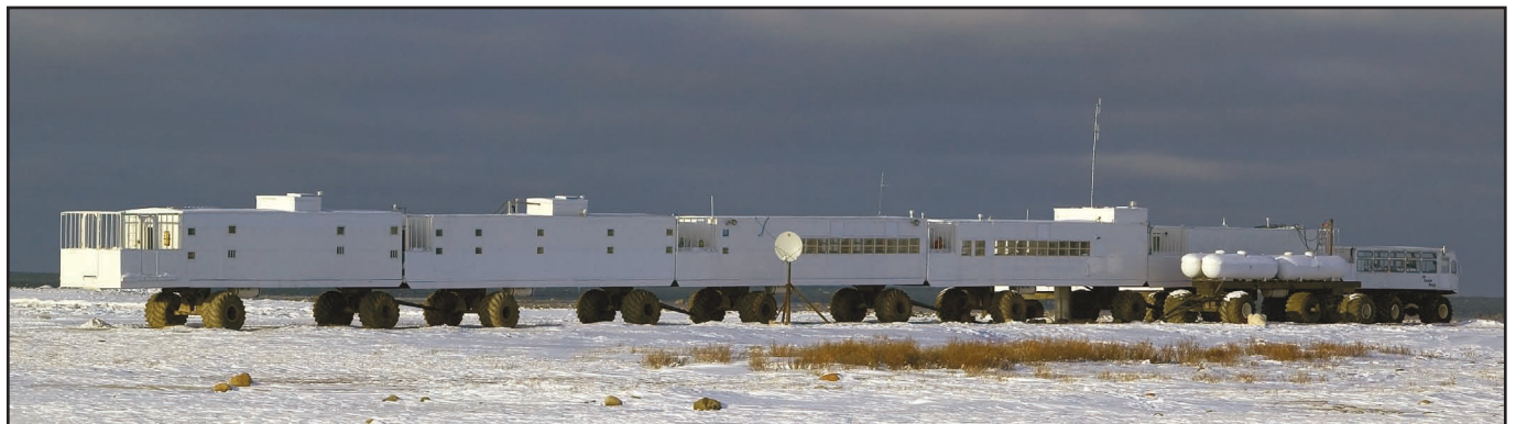
Figure 1—The Tundra Buggy Lodge is an assembly of high-wheeled portable buildings towed out onto the flat, frozen shores of Hudson Bay to accommodate visitors during the October-November polar bear-watching season. The author's antenna stands just to the right of center.
